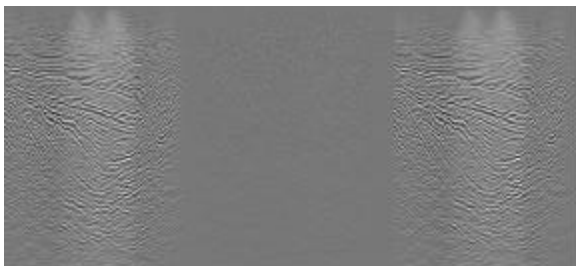
Figure 3. Left panel is migration of uncompressed data (Figure 1), center panel is difference between migration of uncompressed data and 90% compressed data, and third panel is migration of 90% compressed data (Figure 2). The difference is lower amplitude than the images and relatively uncorrelated.
